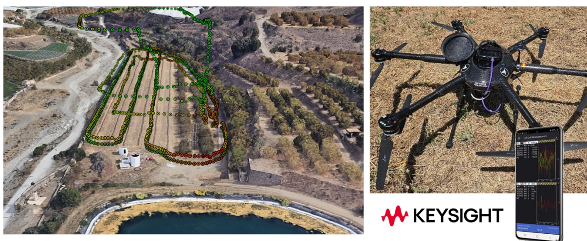
Figure 3-60: Drone-assisted mapping of network coverage at La Mayora
